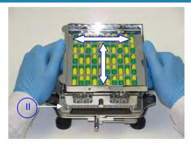
**6.** Repeat Steps 2-5 except in Step 4 place front locating feet of Orienter into holes at position II on Caps Tray. Remove Orienter. If some capsules sit higher than others, gently pat them into place.
