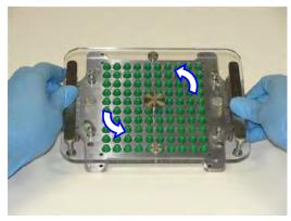
17. Remove Locking Plate by twisting it counter-clockwise. You now have 100 locked capsules. Sometimes for coarse powders, all 100 capsules may re-assemble but not fully lock. If this happens, put the Locking Plate back onto the Caps Tray and continue on to section E.
