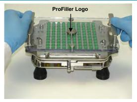
**15.** Remove Powder Tray. Place Caps Tray with Locking Plate onto Filler. ProFiller logo should be right side up.
