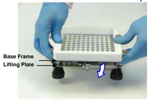
14a. Optionally, pull Cam Lever to gently hold bodies in place. Hold <u>Filler Base</u> <u>Frame</u> and gently tap against table a few times to settle powder. Powder Tray Clamps are recommended when tapping. **DO NOT hold Filler by Lifting Plate** (moveable plate) as capsule bodies will be pushed up out of the filler.
