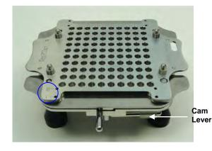
**1.** Place Caps Tray onto Filler with Position I and II markings in front. Check that Cam Lever is set to 3 o'clock.
