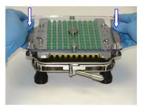
**10.** Push down on Locking Plate handles while lifting up Caps Tray (top metal piece) to separate capsule caps and bodies. Set aside Caps Tray with Locking Plate. See Tip 3. If filling liquids, see Special Fill Materials following these instructions
