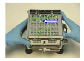
**5.** Push sliding portion of Orienter to the left 1-3 times to drop capsules into Filler, filling every second row. Slide gently to avoid incorrect orientation of capsules. See Tip 2.
