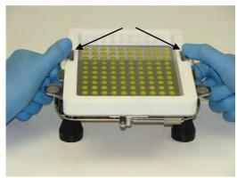
**12.** Place Powder Tray onto Filler. Optionally, attach Powder Tray Clamps. For sticky powders, see Special Fill Materials following these instructions.
