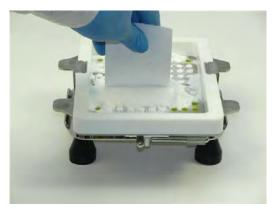
**13.** Pour pre-measured powder onto Filler. Use Powder Spreader to move powder from center towards all 4 edges of Powder Tray frame.
