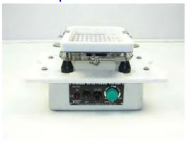
**14c.** Use optional Vibrator as an alternative to or in addition to tamping or tapping (see page 30). Powder Tray Clamps are recommended.
