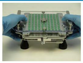
**16.** Press down on clear Locking Plate with thumbs while pulling up Lifting Plate to lock capsules. Do not press on Lifting Plate Handles. Repeat locking with thumbs positioned in different areas of the Locking Plate.
