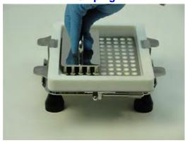
**14.** Use 50-pin Tamper to pack powder. Repeat spreading and tamping as necessary.
