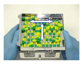
**2.** Pour 50 + capsules onto Orienter. Shake back and forth moving capsules into slots.
