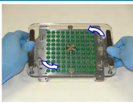
**19.** Flip Caps Tray over. Rotate Locking Plate counterclockwise and remove it. You have 100 filled, locked capsules.
