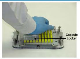
**18.** Remove Caps Tray with Locking Plate and turn them over onto table. Use Capsule Locker to lock capsules. Apply pressure until you feel capsules snap and lock.
