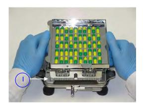
**4.** Place front locating feet of Orienter into holes at position I on Caps Tray.
