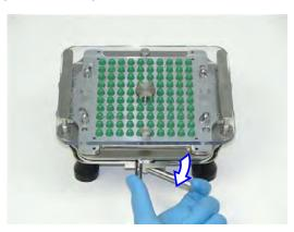
**9.** Gently pull Cam Lever toward the post to secure bodies in Filler. Capsules should be held firmly but should not be squeezed to an oval shape.
