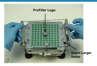
**7.** Hold Locking Plate by handles and place onto Caps Tray by inserting 4 Caps Tray posts into 4 larger holes in Locking Plate. ProFiller logo should be right side up.
