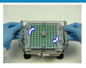
**8.** Hold Locking Plate by handles and twist clockwise to lock into place.
