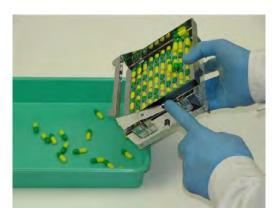
**3.** Tilt Orienter and press tab down to lift gate and pour off excess capsules. See Tip 1.
